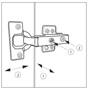
Because these hinges are infinitely adjustable, adjusting one hinge element can sometimes cause the need for adjustments to other elements. But with a few adjustments, you can modify the orientation of the cabinet doors to make sure that they hang perfectly within your cabinet.
