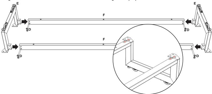
Step 3 - Carefully lay Cabinet C on its back. Using Hex Wrench B1, attach the base assembly to the bottom of the Cabinet C with Screw D and Screw G. \*Note: Each of the metal legs has levelers that can be adjusted
